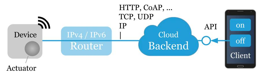
Internet protocols allow a connected device to send data to a backend or to receive commands sent from a client, as shown here, via a backend Web API.
