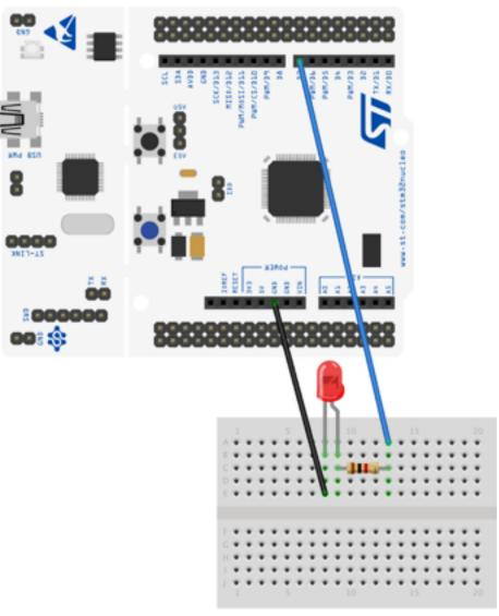
Note: the additional  $1K \Omega$  resistor should be used to prevent damage to the pins / LED if it's reversed
