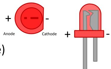
The **LED** (Light Emitting **D**iode) is a simple digital **actuator**.
