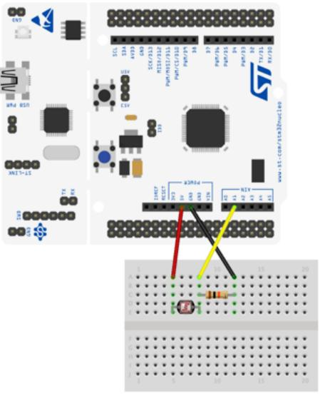
Note: this setup is a voltage-divider, as the 5V total voltage is divided between LDR and resistor to keep 0V < A1 < 2.5V
