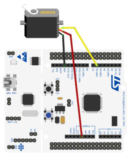
Note: PWM pin D6 is safe to use with the LoRa shield on.
