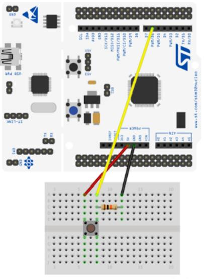
Note: the resistor in this setup is called pull-down 'cause it pulls the pin voltage down to GND (0V) if the switch is open
