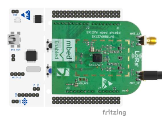
Note: the LoRa shield goes on top of the Nucleo - just make sure the pins line up nicely.
