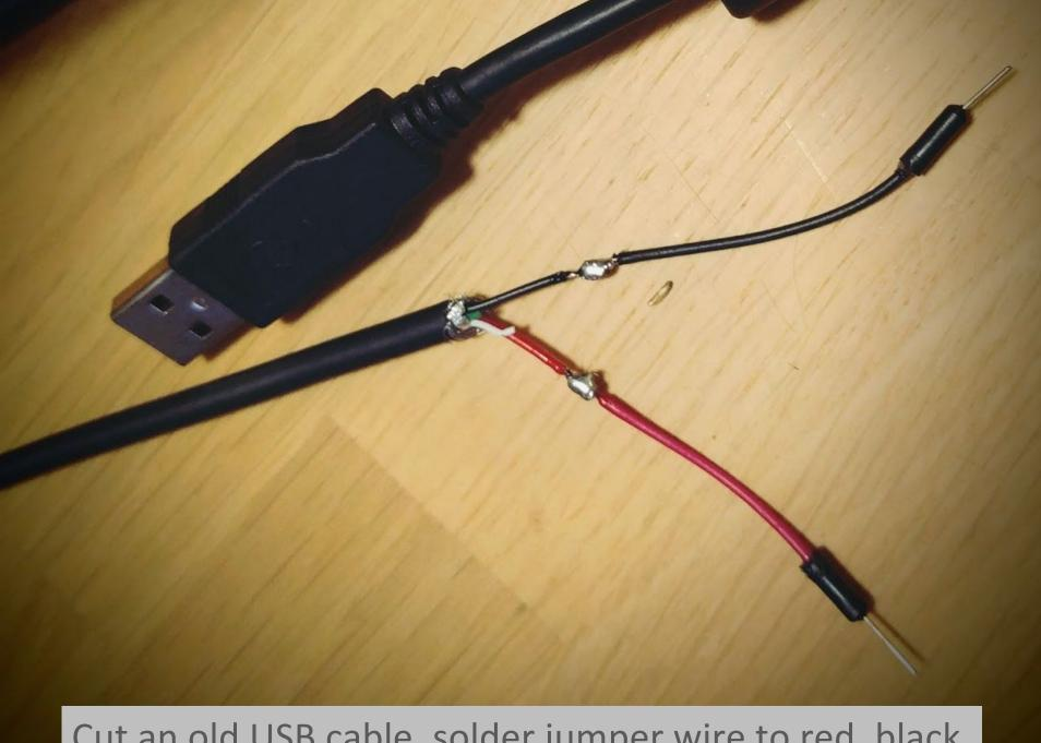
Cut an old USB cable, solder jumper wire to red, black
