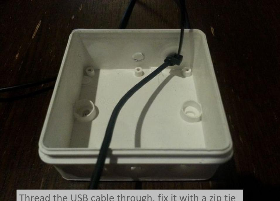
Thread the USB cable through, fix it with a zip tie
