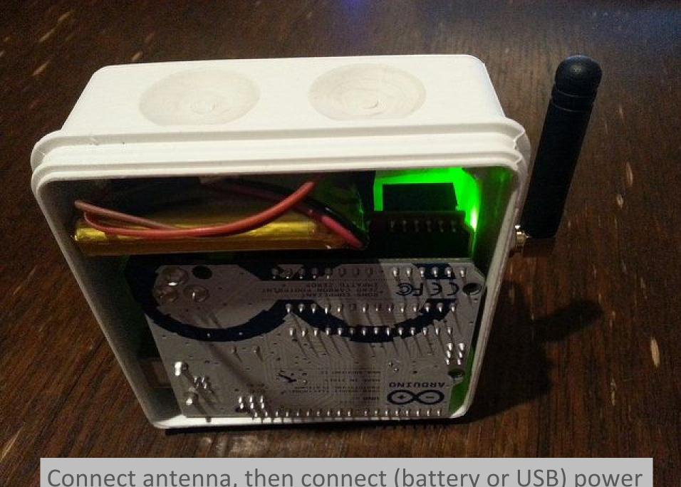
Connect antenna, then connect (battery or USB) power
